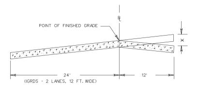
THE PAVEMENT WIDTHS SHOWN IN THE STANDARD TC-5 TABLES ON SHEET 801.20 THROUGH 801.40 REPRESENT TWICE THE DISTANCE FROM THE CROWNLINE TO THE EDGE OF PAVEMENT ON THE HIGH SIDE.
