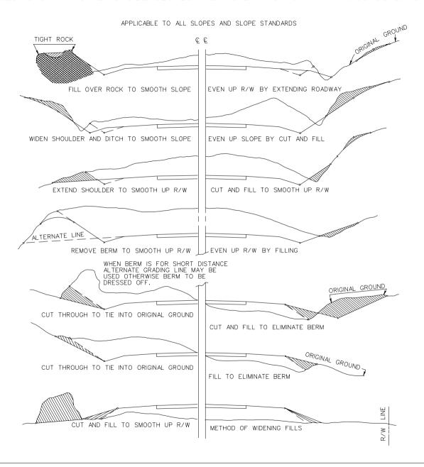
TYPICAL METHODS OF GRADING SIDE SLOPES
