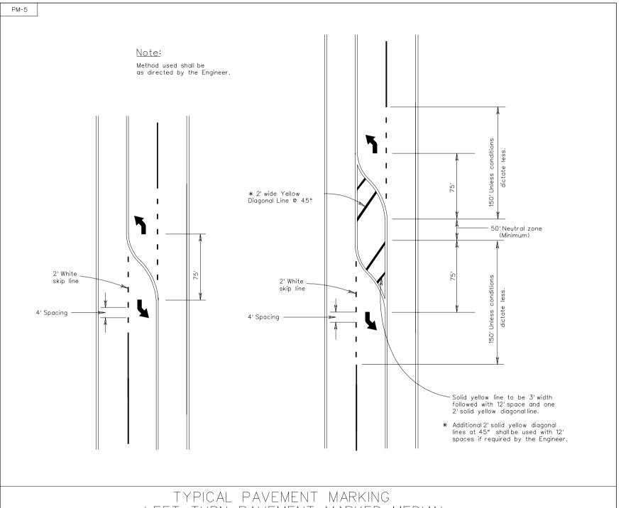
TYPICAL PAVEMENT MARKING LEFT TURN PAVEMENT MARKED MEDIAN
