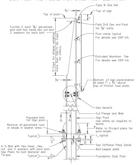
\* Post lengths shown on plans are typical for a 2:1 slope. All post lengths shall be field checked by contractor prior to fabrication.
