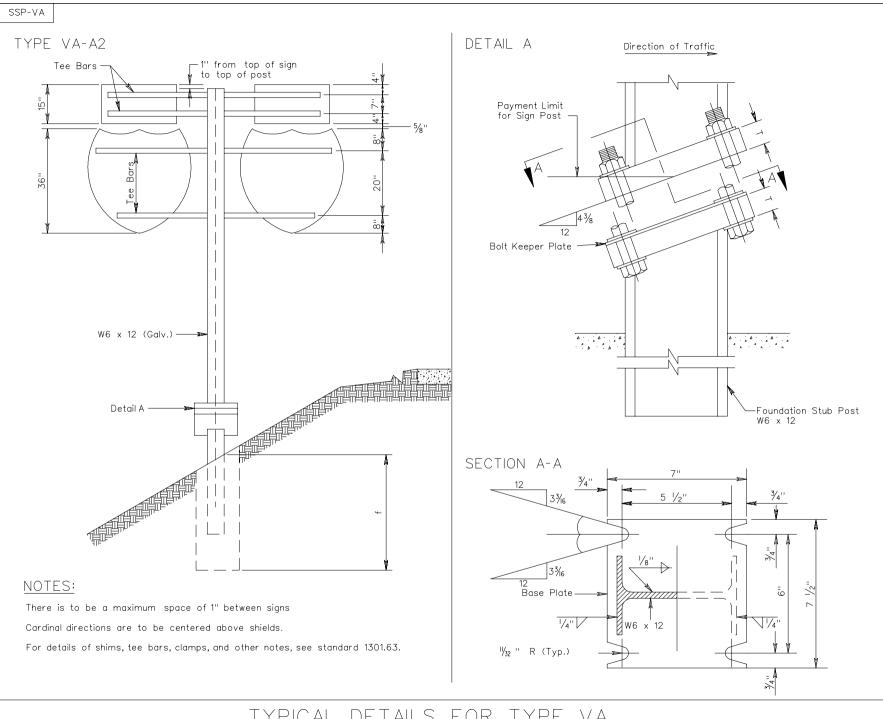
TYPICAL DETAILS FOR TYPE VA SIGN STRUCTURES
