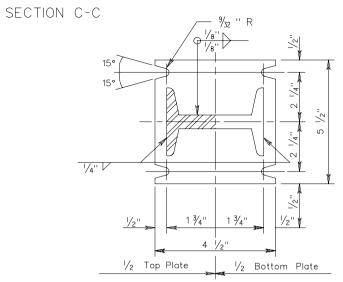
For Type VA-A, use  $\frac{1}{2}$ " Diameter High Strength Bolts with Hex Head, Hex Nut and 3 Washers each Stainless Steel or ASTM A325. Bolts to be installed with a torque of 155 inch lbs. for typical assembly, see Project Plans.
