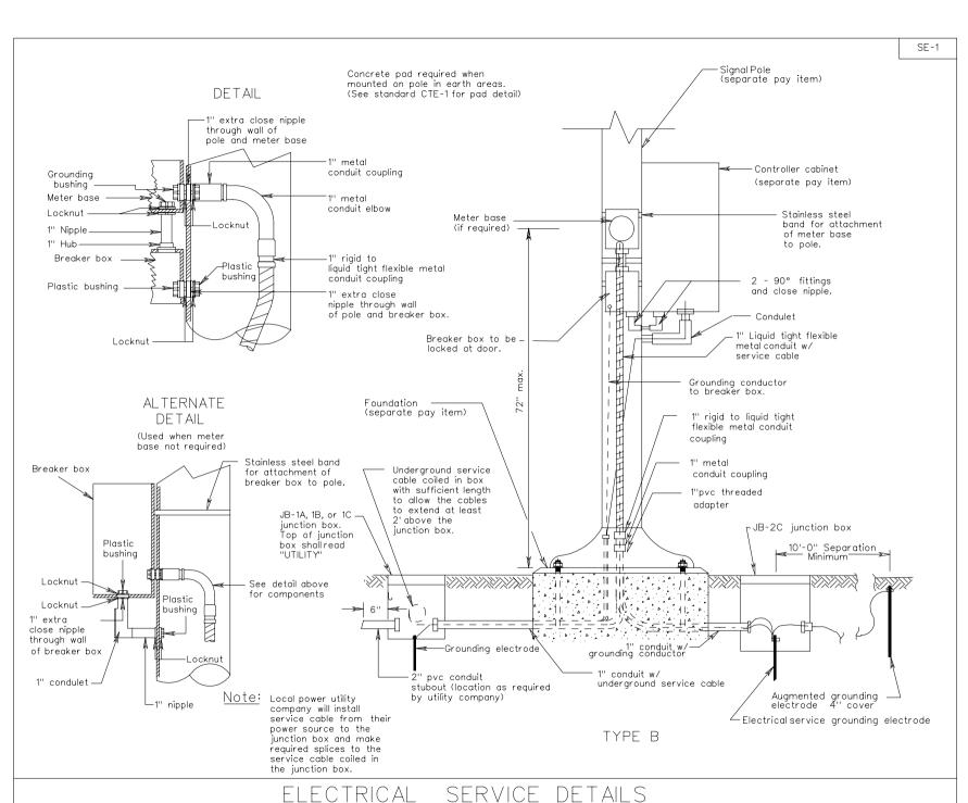
ELECTRICAL SERVICE DETAILS SIGNAL INSTALLATION
