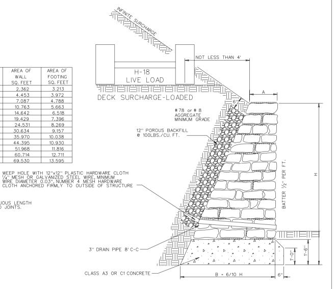
DRAIN PIPES ARE TO BE ONE CONTINUOUS LENGTH OR BELL AND SPIGOT WITH MORTARED JOINTS.
