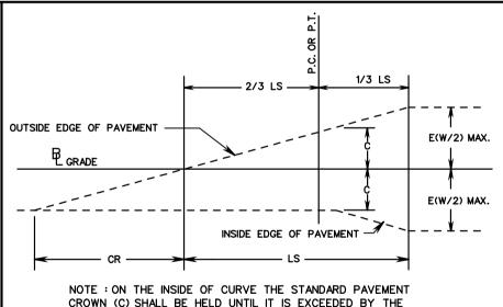
CROWN (C) SHALL BE HELD UNTIL IT IS EXCEEDED BY THE TABULATED RATE OF SUPERELEVATION (E).
