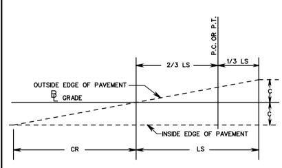
SUPERELEVATED BY AN AMOUNT EQUAL TO THE STANDARD PAVEMENT CROWN
