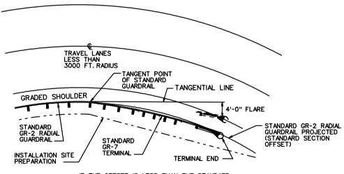
IF THE OFFSET IS LESS THAN THE STANDARD SECTION OFFSET THE OFFSET WILL BE HELD AT THE STANDARD SECTION OFFSET.
