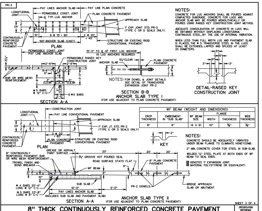
8" THICK CONTINUOUSLY REINFORCED CONCRETE PAVEMENT (FOR USE WITH BAR OR WIRE MESH REINFORCEMENT)
