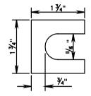
Furnish 2 @ .063" thick and 2 @ .032" thick shims per post. Shims shall be fabricated from brass conforming to ASTM B36 or from stainless steel with a minimum chromium content of 11.50%. No more than 2 shims shall be used per bolt with a maximum of 4 shims per post.
