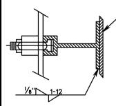
Attach sign to tee bar by using 1100-H18 aluminum alloy 1/4" - 20 x 1/2" long studs electrically welded to back of sign panel by the Capacitor Discharge Method. Maximum horizontal spacing of studs shall be on 6" centers beginning 1" from each end of tee bar. 7075-T6 aluminum alloy spring lockwasher 0.255" I.D. x 0.493" 0.D. x 0.062" thick shall be provided for each stud. 6262-T9 aluminum alloy 1/4" - 20 hexagon head nut, torque to 25 in lbs. shall be provided for each stud.
