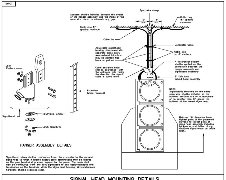
SIGNAL HEAD MOUNTING DETAILS SPAN WIRE
