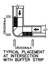
THE SELECTION OF CURB TYPE AND THE CONFIGURATION OF THE UTILITY STRIP MAY VARY TO MEET EXISTING FIELD CONDITIONS AND ROADWAY GEOMETRICS PROVIDING THE DIMINSIONS AND SLOPES ARE AS NOTED.
