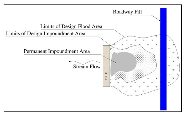
Example 3 Roadway causeway within the Design Flood Area but outside the limits of the Design Impoundment Area. Causeway is not treated as a dam.
