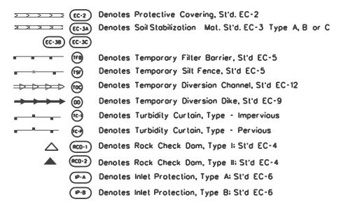
The ESC symbols are to be used to denote proposed erosion and sediment control items on the plans and are available in the CADD Cell and Custom Line Style Libraries and the GeoPak Road Plan View Labels.
