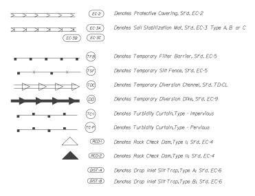
The ESC symbols are to be used to denote proposed erosion and sediment control items on the plans and are available in the CADD Cell and Custom Line Style Libraries and the GeoPak Road Plan View Labels.
