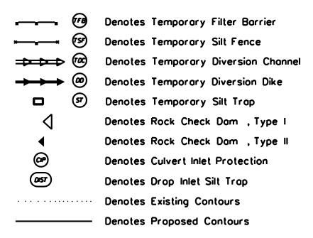
• The previous symbols are to be used to denote erosion control items and are available as CADD cells. The following note is to be placed on level 63 of all applicable plan sheets (cell name: ESNOTE1):
