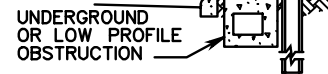
SECTION D-D DETAIL OF MULTIPLE BLOCK-OUT TO AVOID UNDERGROUND OR LOW PROFILE OBSTRUCTION
