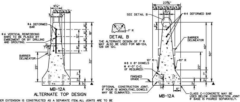
IF BARRIER EXTENSION IS CONSTRUCTED AS A SEPARATE ITEM, ALL JOINTS ARE TO BE CONSTRUCTED AT THE SAME INTERVAL AS CONCRETE BARRIER. ALL VERTICAL BARS ARE #4 AT 24" MAX. SPACING. LENGTH OF DOWELS SHALL BE 20". VERTICAL BARS MAY BE PLACED IN THE CONCRETE OR BONDED INTO DRILLED HOLES IN HARDENED CONCRETE. WHEN HOLES ARE DRILLED NON-SHRINK GROUT SHALL BE USED TO BOND THE BARS IN PLACE.
