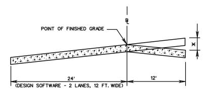
THE PAVEMENT WIDTHS SHOWN IN THE STANDARD TC-5.01 TABLES ON SHEET 802.24 THROUGH 802.42 REPRESENT TWICE THE DISTANCE FROM THE CROWNLINE TO THE EDGE OF PAVEMENT ON THE HIGH SIDE.
