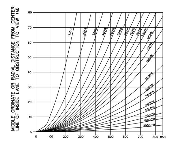
\* 2.0 FEET STOPPING 3.5 FEET PASSING LINE OF SIGHT AT MID POINT TO BE 2.0' ABOVE EDGE OF PAVE-MENT FOR STOPPING SIGHT DISTANCE, AND 4.0' FOR PASS-ING SIGHT DISTANCE.
