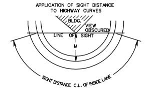
LENGTH OF ARC SUBTENDED OR CLEAR SIGHT DISTANCE MEASURED ALONG CENTER LINE OF INSIDE LANE (S)
