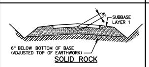
REMOVE ROCK TO A POINT 6" BELOW BOTTOM OF BASE FOR ENTIRE WIDTH OF ROADWAY. BACKFILL WITH SUBBASE LAYER 1 USING BOTTOM 2" AS A LEVELING COURSE.
