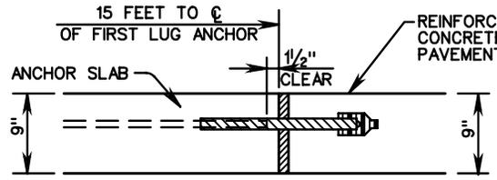
SECTION E-E ANCHOR SLAB TYPE I
