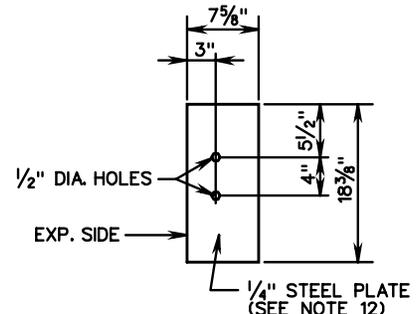
ANCHOR SLAB TYPE II END PLATE DETAIL
