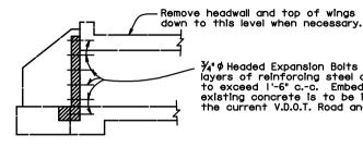
7/4" \psi Headed Expansion Bolts placed between layers of reinforcing steel at a spacing not to exceed 1'-6" c.-c. Embedment into new and existing concrete is to be in accordance with the current V.D.O.T. Road and Bridge Specifications.
