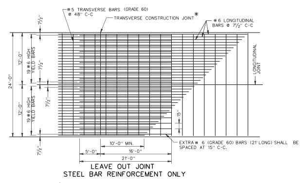
st longitudinal steel to continue through joint.
