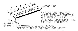
DETAIL FOR LOCATION OF EDGE LINES ON CURB SECTIONS OF ROADWAY (NO GUTTER)
