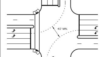
DETAIL FOR DOTTED EXTENSION THROUGH INTERSECTION AT DUAL TURN LANES
