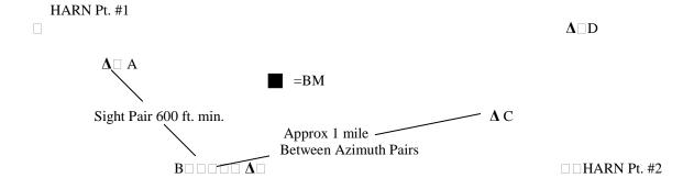
A,B,C,D = VDOT Route Survey Control Points; Coordinates to be Determined HARN #1 to HARN #2 = 17 km = BM on NAVD88 datum; GDOP = 2.5; 6 Satellites HARN Points Have Known X, Y & Z Values
