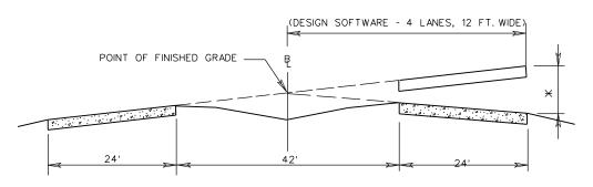
X THE ELEVATION DIFFERENTIAL BETWEEN NORMAL CROWN AND MAXIMUM SUPERELEVATION, RELATIVE TO THE BASELINE PROFILE.
