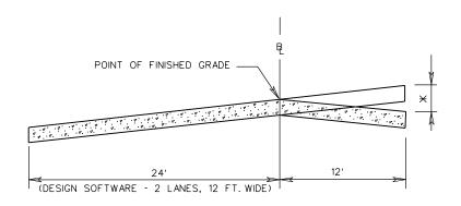
THE PAVEMENT WIDTHS SHOWN IN THE STANDARD TC-5.11 TABLES ON SHEET 803.24 THROUGH 803.44 REPRESENT TWICE THE DISTANCE FROM THE CROWNLINE TO THE EDGE OF PAVEMENT ON THE HIGH SIDE.
