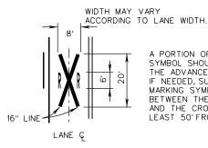
A PORTION OF THE PAVEMENT MARKING SYMBOL SHOULD BE DIRECTLY OPPOSITE THE ADVANCE WARNING SIGN (W10-1). IF NEEDED, SUPPLEMENTAL PAVEMENT MARKING SYMBOLS MAY BE PLACED BY THE ADVANCE WARNING SIGN AND THE CROSSING, BUT SHOULD BE AT LEAST 50'FROM THE STOP OR YIELD LINE.
