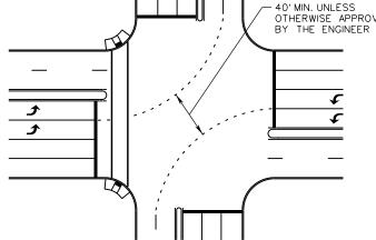
DETAIL FOR DOTTED EXTENSION THROUGH INTERSECTION AT DUAL TURN LANES
