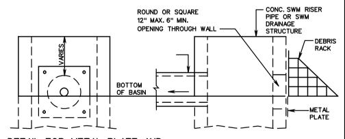
DETAIL FOR METAL PLATE AND SIDE VIEW WITH DEBRIS RACK WATER QUALITY ORIFICE
